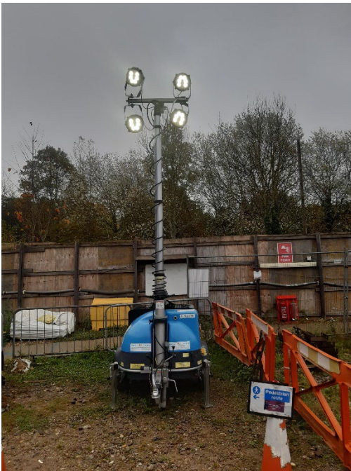
Figure 4 - Ecolite-TH200 Lighting Tower
