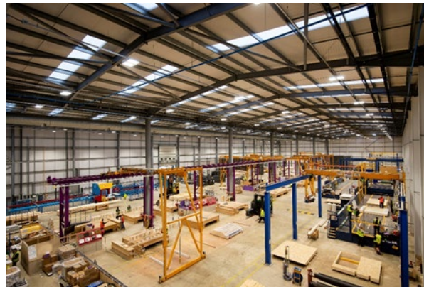
Figure 1 - Fabricating SIP's panels
